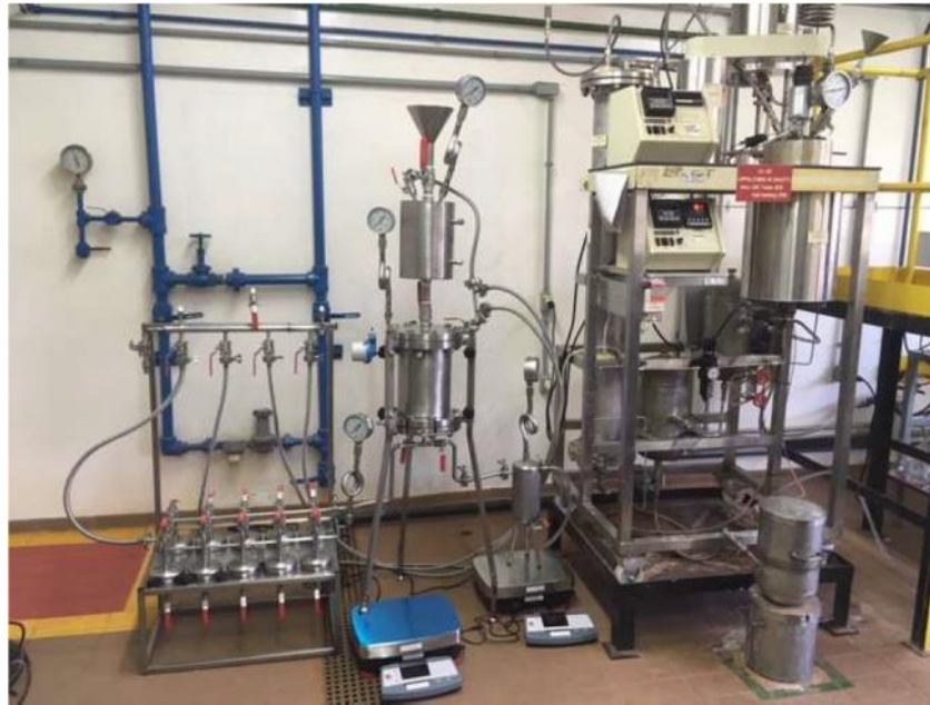
Figure 1. Autoclave apparatus (right) and pressure filter (left) in the B&A R&D laboratory [6].
